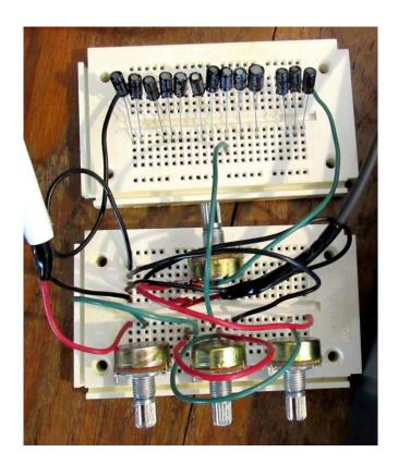
This component can create a quasi-AD envelope (gate) at Output 1 or a quasi-D envelop (trigger) at Output 2. This can be selected by the connection represented by S1 in the diagram, realized as changing the jumper connection.
